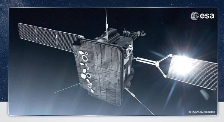
The METIS project (The Multi-Element Telescope for Imaging and Spectroscopy) is one of ten main experiments on the Solar Orbiter satellite to be launched to the Sun in 2018. The Solar Orbiter will come unprecedentedly close to our parent star, to a distance of 42 million kilometres and the 25° slope of the satellite to the Equator will allow us to explore even the less known solar pole regions.
